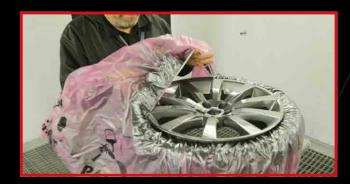
STEP 5 Remove the mask after bake cycle. Remove masking tape from valve and Advanced Foam Masking Tape from bolt holes.
