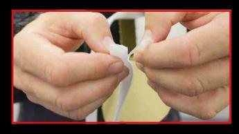
**STEP 2**Remove the release liner exposing the adhesive.
