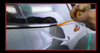
**STEP 3**Remove, leaving no adhesive residue.
