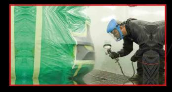
STEP 5 Apply base coat and clearcoat.
