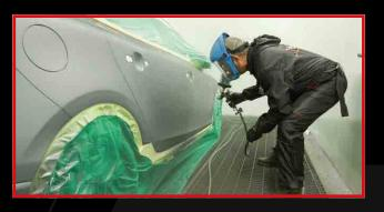
Apply base coat, flash-off, then apply clearcoat.
