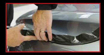
STEP 1 Apply to the area requiring protection from sanding.
