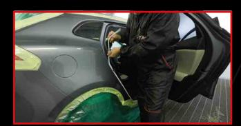
**STEP 5**Stretch to cleanly remove, leaving no adhesive residue.
