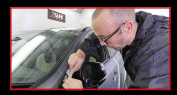
**STEP 3**Pull the rubber down and away from the panel.
