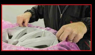
STEP 2 Unwrap a mask and use the elasticated centre for precise positioning on the wheel/rim.
