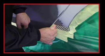
**STEP 1** Apply directly to masked area prior to base coat.
