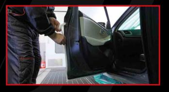
STEP 6 Stretch to remove leaving no residue.
