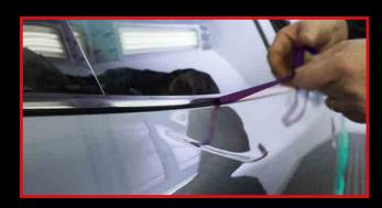
STEP 3 Remove, leaving no adhesive residue.
