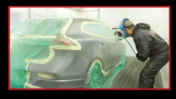
**STEP 2**Mask off as normal and apply basecoat and clearcoat.
