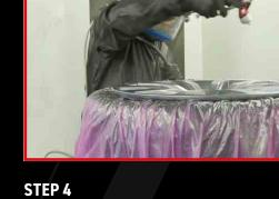
Use 1011 Advanced Foam Masking Tape to plug bolt holes and masking tape over the valve, then apply primer, base coat and clearcoat.
