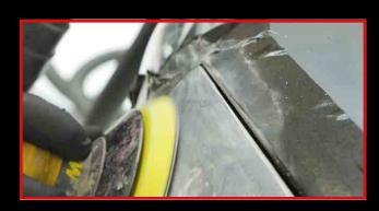
STEP 3 Sand over required area with the tape protecting the adjacent panel.
