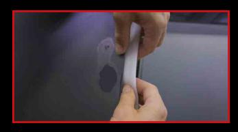
STEP 1 Apply the tape to the moving part, ensuring the adhesive is hidden.
