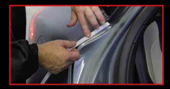
**STEP 1**Following the contours, apply to the panel being careful not to stretch the tape.
