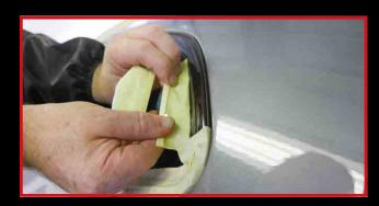
STEP 3 Allow paint to dry and remove all masking materials.
