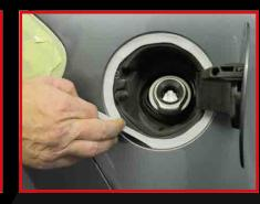
**STEP 3**Remove by stretching once clearcoat has been baked.
