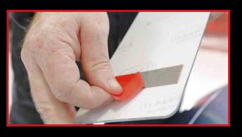
**STEP 2**Remove the protective release liner.
