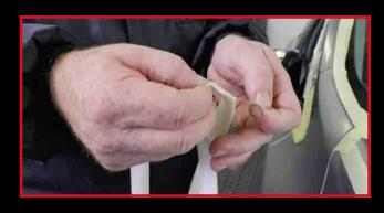
**STEP 2**Remove the liner to expose the adhesive.
