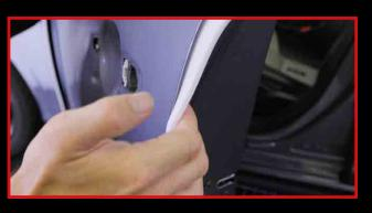
STEP 2 Apply pressure to the adhesive side.
