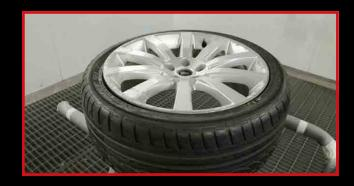
STEP 1 Deflate the tyre and break the bead.
