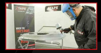
**STEP 4**Apply primer, baseboat and clearcoat immediately with no curing time or need for adhesion promoter.
