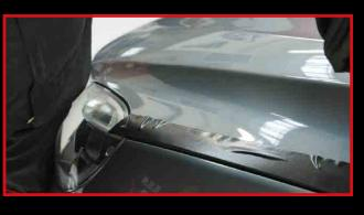
STEP 2 Apply pressure to secure the tape into place.
