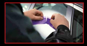
**STEP 1**Measure the section required and easily tear small sections using perforations.
