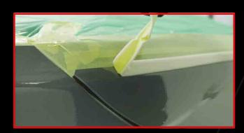
**STEP 5**Where possible, remove while clearcoat is wet.
