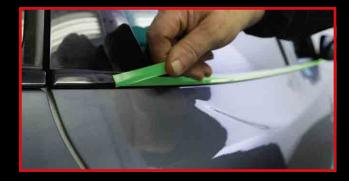
STEP 3 Remove, leaving no adhesive residue.
