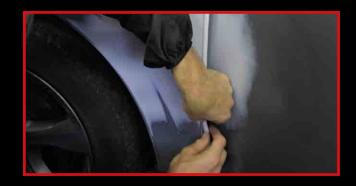
Apply to the back of the moving part (or the fixed part for the A-Pillar), hiding the adhesive and leaving the non-adhesive section extended.
